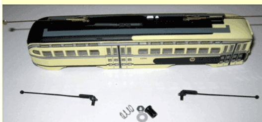
Figure 5 - Bowser 1250 poles installed with extra 1250 hardware shown.
