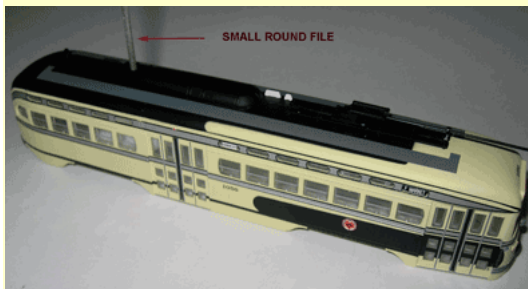
Figure 4 - Filing out the holes in the roof for the trolley pole.
